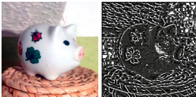
Fig. 4. On the left is the input image, and on the right are extracted LBP_{8,3}^i features.
