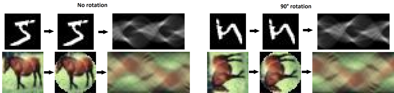
Fig. 2. Radon transform calculation. The images (examples taken from MNIST and CIFAR-10 datasets) are masked by the inscribed circle. Then, their Radon transform is computed. Image rotation results in a cyclic shift of the Radon transform along the horizontal axis.
