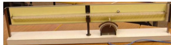
Fig. 1. Laboratory model 'ball on rod'.
